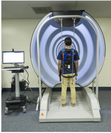
Fig. 1. Subjects stood still on a forceplate with their feet positioned according to a standardized grid and arms by the side. During the assessment, subjects looked forward with open eyes fixed on a target 1 meter in front of them.
